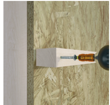
Mounting of installation level
